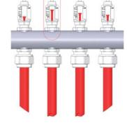
Turn the valve adjustment knob to bring the value of the selected branch flow to the desired value.
