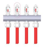
Then act on the adjustment of the manifold valves to vary the flow rate of the other branches.
